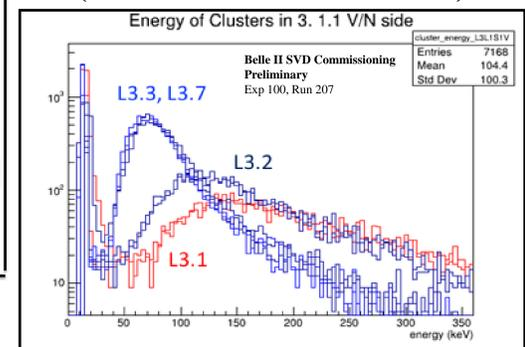
Distribution of the energy deposit in a horizontal silicon sensor ( $t=300\mu\text{m}$ ) by a cosmic ray ( $\sim$ MIP) is peaking at 80keV. The deposit distribution for random-trigger events was peaking at  $\sim$ 20keV.
