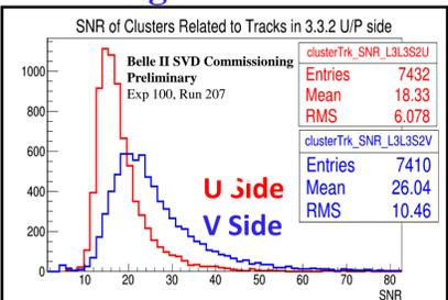
S/N greater than 20, with the N side performing slightly better than the P side, as expected.
