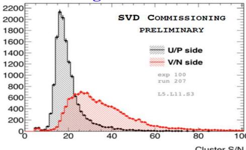
The S/N ratio is larger than 25 for N side, slightly lower on P side due to the longer strips and larger capacitance load to the preamplifier.
