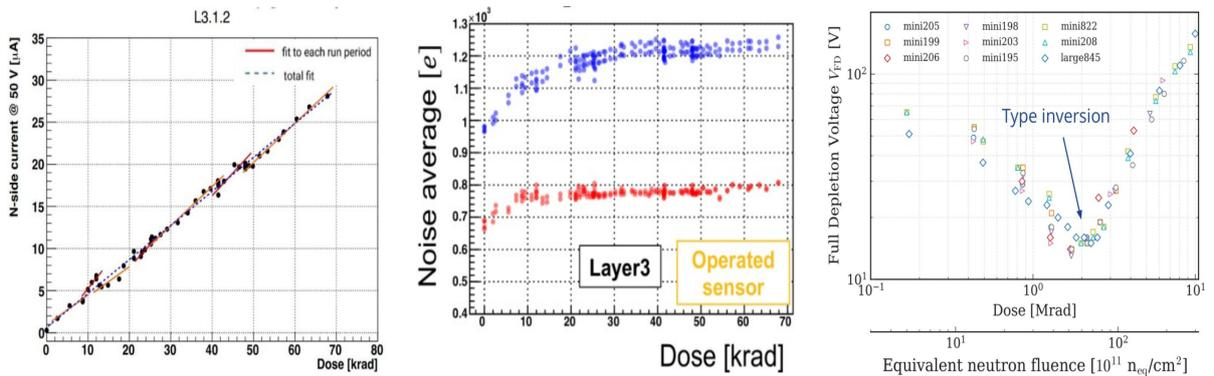
**Figure 4:** Left plot: Leakage current as a function of the accumulated dose; Center plot: the average noise level as a function of accumulated dose for p-side (blue dots) and n-side (red dots); Right plot: full depletion voltage as a function of the accumulated dose with the type inversion observed at 2 Mrad.
