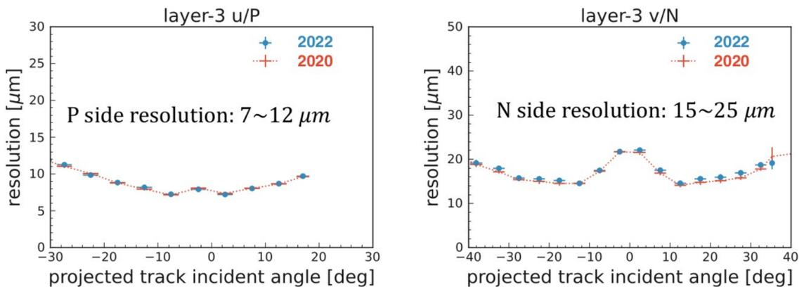
**Figure 3:** Distribution of position resolution for p-side (left) and n-side (right) as a function of the incident angle. Comparison between data taken in 2020 (dots) and 2022 (dotted line) is presented.
