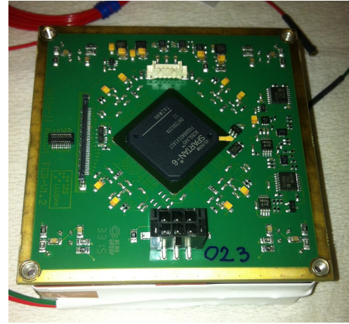
Figure 2: Photo of the front-end board attached to HAPD. There are three connector cables for a data transfer, board and bias power supplies
