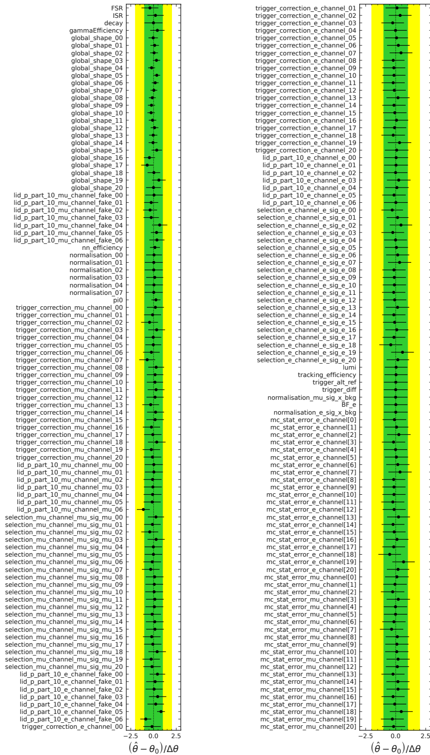
Figure 5.30: The pull plot for the 2-channel fit, showing all nuisance parameters with names as described in Table 4.26. The black marker indicates the pull value, and the error bar shows the post-fit uncertainties of the nuisance parameters. None of the parameters has a pull value that deviates significantly from zero.
