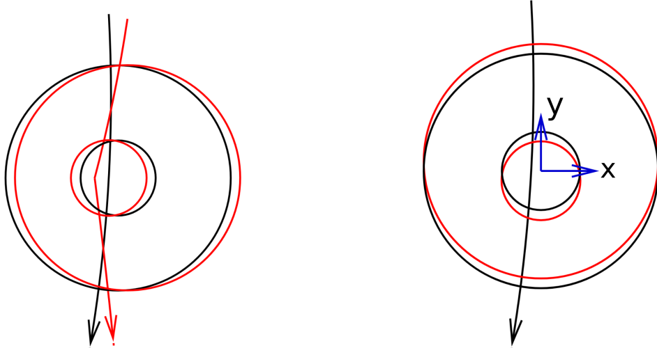
Figure 15.5: Illustration of the off-centering in the y -direction (right) to which cosmic ray tracks (mostly vertical) are poorly sensitive. For the off-centering in the x -direction (left), this distortion creates a kink in the (merged) cosmic trajectory, which makes it resolvable by the alignment to much better precision. [81]
