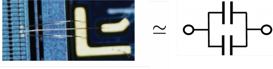
Figure 4.5: Example of the wire bonding for C_{\text{int}} measurement, wire bonded on the DC pad of each strip. There are three strips as one pair to measure C_{\text{int}} , the center strip and two adjacent strips are connecting different signal terminals via the protection circuit leading to an LCR meter. Thus, the equivalent electrical circuit is two capacitors (two interstrip capacitances) connected in parallel (right figure).
