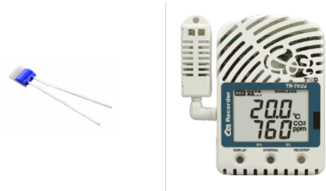
Figure 4.14: Thermometer for checking environment temperature around sensor: Pt100 (left), TR-76Ui by T&D Corporation (right)
