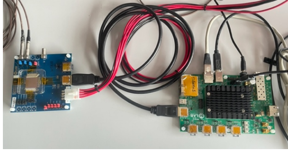
Figure 5.3: Test setup for TJ-Monopix2 using the BDAQ53 system.
