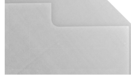
Microchannels seen with X-ray of the cooling plate
