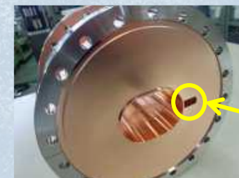
Beam channel for injection
