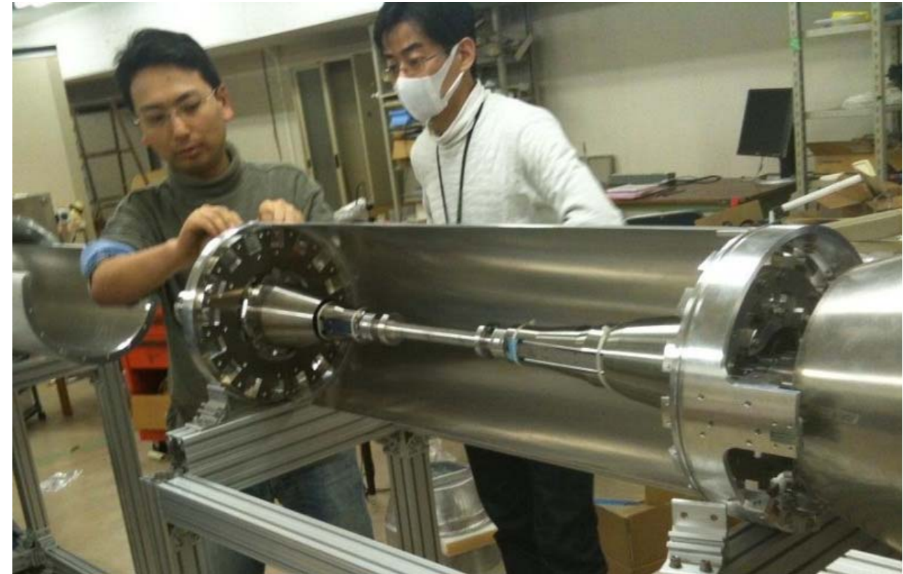
beryllium beam pipe at interaction point
