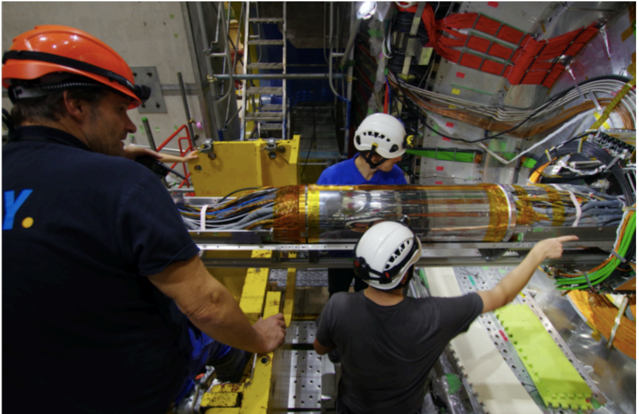
Pixel Detector (PXD): Layer 1 and partial Layer 2 Silicon-strip Vertex Detector (SVD): all 4 layers
