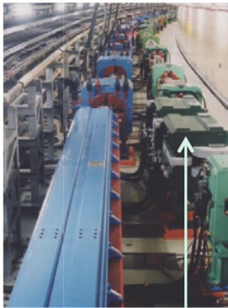
Replace short dipoles with longer ones (LER)
