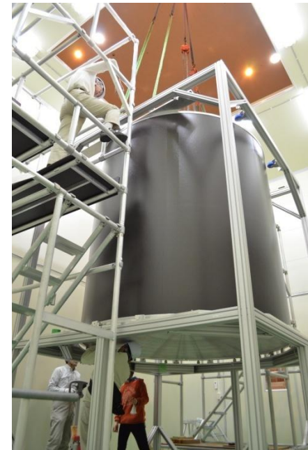
Wire stringing in a clean room in Fuji Hall
