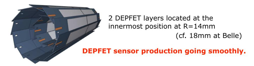
(Successful test beam in 2014 with PXD and SVD Prototypes): To reduce 20 Gbit/s data from PXD, read out **Regions Of Interest** from projected SVD tracks
