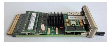
Figure 4.5: Photograph of the xFP AMC card equipped with a cooling block on top the FPGA and two DDR2 SO-DIMM modules.
