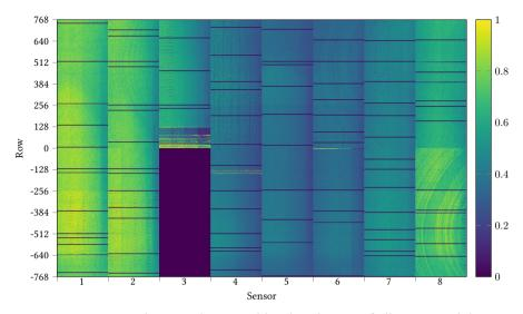
Figure 6.8: Hitmaps showing the typical hit distribution of all inner modules in a single run. Artifacts are explained in the text. Forward modules are at the top, while backward modules are at the bottom. Sensor 1 is located in the +X direction, which points to the outside of the accelerator tunnel.
