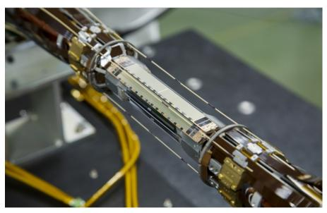
Figure 3.7: Photograph of the mounted PXD.
