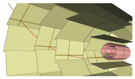
Figure 4.3: Illustration of ROI calculation. A charged particle moves outward on a helical trajectory from the interaction point on the active surface of the PXD and half of the SVD layer, leaving hits in each strip of the SVD. As a result, a particle's track can be reconstructed, and the two PXD layers are extrapolated to determine the most likely intercept locations. Regions of interest around those intercept locations are defined.
