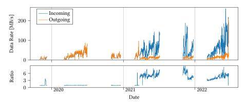
Figure 6.2: Comparison between input and output data rates of ONSEN averaged for each physics run. The highest input data rate was reached near the end at peak luminosity in 2022 with over 250 MB/s. In the lower part the fraction is shown. During 2021 the *event filtering* was enabled, which results in a permanent increase of the ratio.
