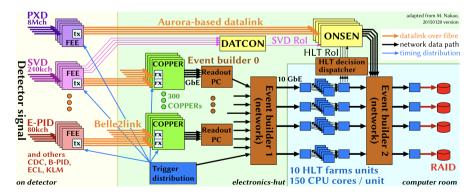
Figure 4.1: Overview of the Belle II data acquisition system.
