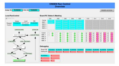
Figure 5.5: State diagram of the ONSEN run control with stable and transition states. The current state is based on all subsystems, each possible to define individual criteria, and the requested state from Belle II. In this example the current state is RUNNING indicating active data acquisition. Colors are used for each state for better visualization for the shifter. On the right all subsystems (CNCB and xFP) are shown with their own RC state.
