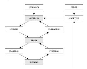
Figure 5.10: State diagram of the run control with possible request states in gray and additional transition states. The ERROR state can be entered for all states.
