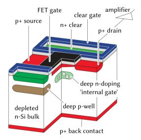
Figure 3.8: Illustration of a single DEPFET pixel.
