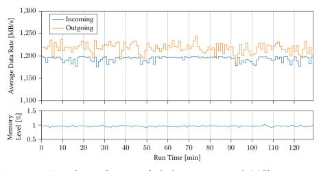
Figure 6.4: First 2 hours of runtime of a high rate test run with 0.3% occupancy test pattern at 30 kHz. With a maximum delay of 300 ms between arrival of DHH and HLT data, the memory fill level stays at 1%. The fill level may be different with higher input rates and filtering.
