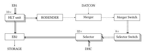
Figure 4.6: Schematic of the connectivity of ONSEN. Each HLT unit receives detector data from EB1 and calculates ROIs for each event. At first the ROI information is sent to the Merger, where ROIs are combined with DATCON ones. Afterwards the merged ROIs are distributed to each Selector as indicated by the dashed lines. After processing the DHC data, the Selector sends the reduced pixel data to EB2, where it is merged with the rest of the data before being stored.
