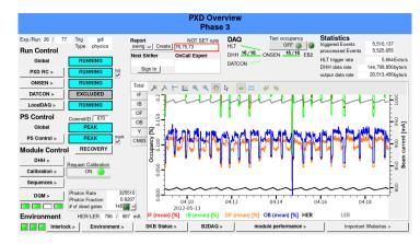
Figure 5.1: Main operator interface for the PXD, providing helpful information like the average occupancy seen in each module, the status of the power supplies and the data acquisition system. Buttons allow to navigate to further views to get more detailed information for shifter and experts.
