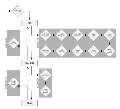
Figure 5.9: State diagram of the DHH Sequence. The rectangles represent persistent states, the diamond shapes transition states. The double arrow transitions require a new requested state. The inverse way is also possible, but nearly without any action. A transition from every state to an ERROR state is possible in case the desired action failed or the connection to the IOC or hardware failed.
