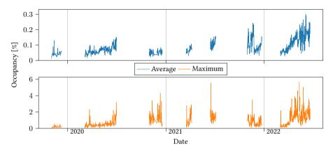
Figure 6.7: Average and maximum occupancy for each run in Phase 3. The PXD DAQ is designed to handle up to  $2.5\,\%$  average occupancy.
