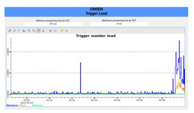
Figure 5.4: The trigger lead is the difference between the trigger number of the pixel data and the trigger number of the ROI data. Since all Selector nodes run independently the EPICS PVs are not published synchronously and differences are possible. Therefore the maximum, minimum and mean of the differences are calculated. The minimum value is divided by the trigger rate to estimate the minimum time interval.
