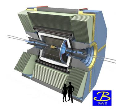
Figure 3.3: Sketch of the Belle II detector. Each subdetector is colorized differently. From the outmost KLM in green, followed by the solenoid coil and the ECL in white, the ARICH in blue tiles in the forward region, the TOP as transparent slabs, the CDC as grey long strips and the VXD, which is in yellow for the SVD and in red for the PXD subsystem.
