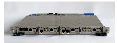
Figure 4.4: Photograph of the CNCB with 4 xFP cards installed. The plate on top ensure air flow when installed in the ATCA shelf.
