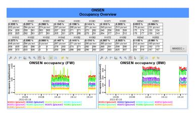
Figure 5.3: Calculation of average pixel per event per module over multiple Selector nodes. The average occupancy results from dividing by the maximum number of pixels per module (192 000). The plots are divided into forward and backward modules. The fluctuations for all modules are caused by the injection pattern of the accelerator.
