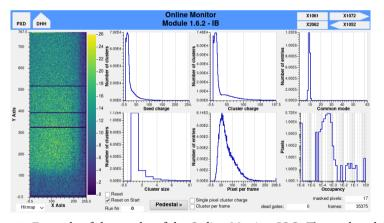
Figure 5.12: Example of the results of the Online Monitor IOC. The analyzed data is presented as PVs and are visible for the PXD shifter. By default the histograms are reset for each run and the hitmaps are included in the online logbook entry created by the local DAQ control IOC.
