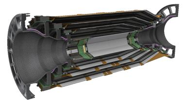
Figure 3.5: A 3D model of the SVD. In boost direction the sensor have a wedge shape in order to increase the angular coverage to 17°.
