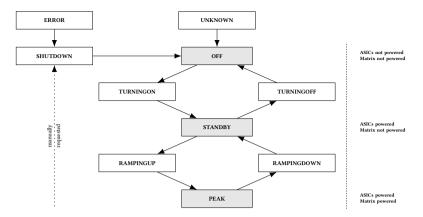
Figure 5.7: State diagram of the PS control with possible request states in gray and additional transition states. On the left side the meaning of the corresponding stable state is given.
