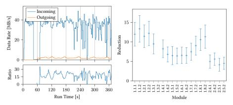
Figure 6.3: Single run with ROI filtering enabled. In the lower part the fraction is shown. The high fluctuations arise from the level-1 trigger, e.g. when a subsystem is busy and additional triggers are rejected. The right plot shows the total reduction ratio for ROI filtering only for each module individually calculated by DQM. The error bars represent the standard deviation.
