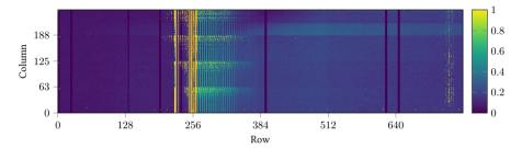
Figure 6.6: Hitmap of module 1.1.2 during a single run. The values are clipped at the 98th percentile to reveal the remaining hits. The occupancy of this module was roughly 8 times higher than other modules. Only the first 100 000 events are included. The ticks on both axes mark the geometrical borders of the ASICs. Similar behavior was also observed in other modules due to persistent radiation damage.
