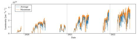
Figure 6.1: Luminosity of each longer run in Phase 3 detected by ECL. In June 2022 the instantaneous luminosity record of  $4.71 \times 10^{34}$  cm<sup>-2</sup> s<sup>-1</sup> was reached [23]. Several plots in this chapter are made using the same time period, allowing for a correlation between the different statistics and the luminosity.
