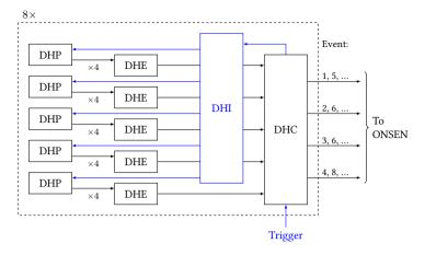
Figure 4.2: Schematic of the connectivity of DHH. The DHC is the central system, which forwards the trigger signal via the DHI to the modules. Afterwards the data is sent from the DHPs mounted on the module to the DHEs and the DHCs. The DHE and DHC perform subevent building. Each DHC sends events to four ONSEN nodes using a round robin scheme.
