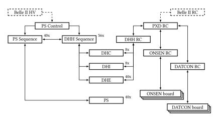
Figure 5.6: Overview of the PXD IOCs and their connectivity. There any many smaller IOCs available and the counter next to an IOC does not necessarily represent the number of actual applications started on a server. This schematic focuses on the IOCs with highest priority and are essential for the minimal operation.
