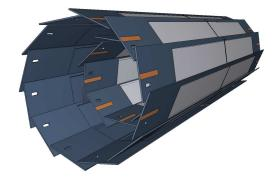
Figure 3.4: Scheme of the PXD detector geometry.
