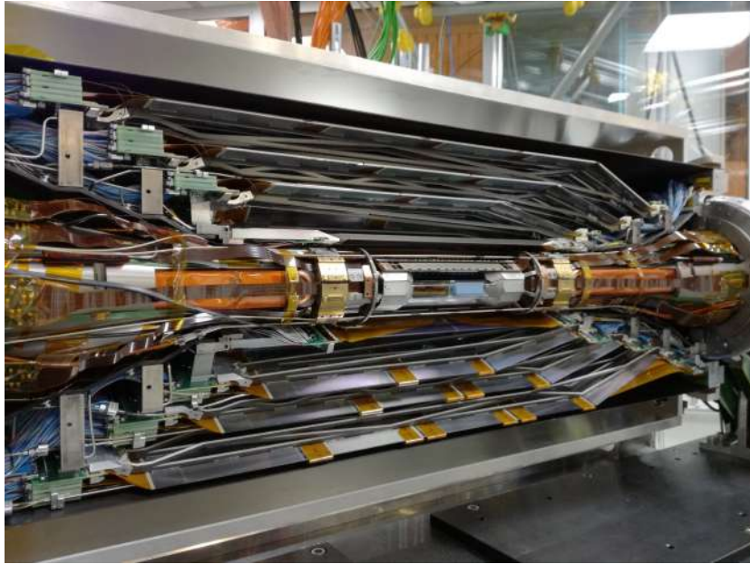
Figure 3.4: The Belle II SVD already matched with the PXD and ready to be installed in at the Interaction Point of the detector (December 2018).
