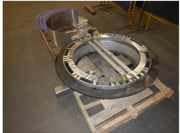
(d) Forward shield braces prior to lead casting.
