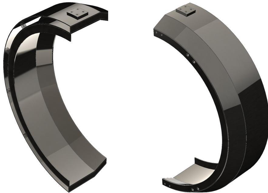
Figure D.4: Geometry of the shells of the backward shield
