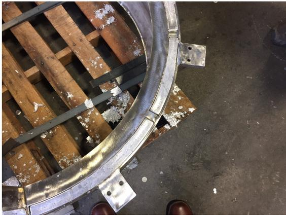
(c) Backward shield after lead casting.
