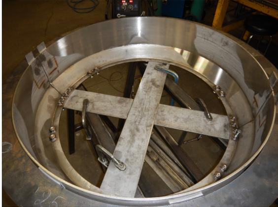
(a) Backward shield during shell welding.
