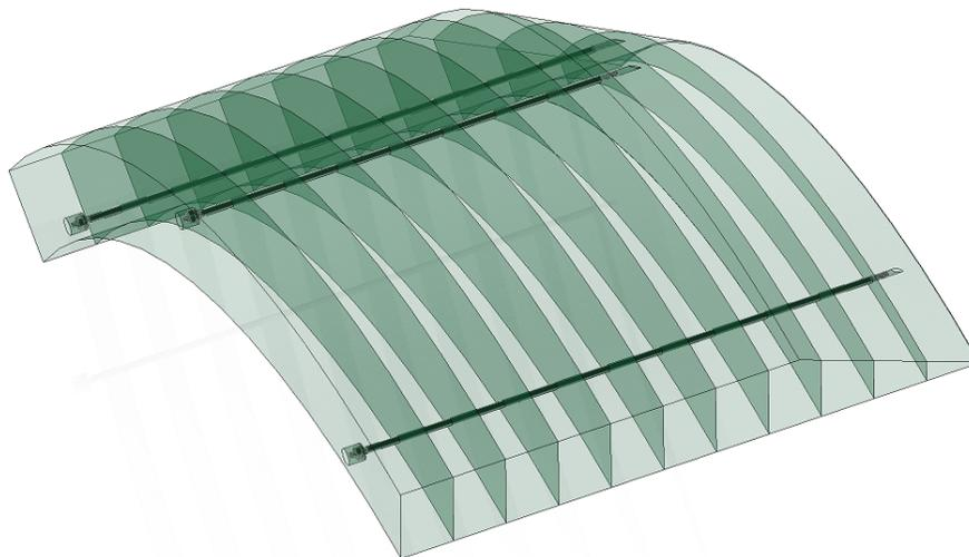
Figure D.8: Geometry of a backward neutron absorber sub-assembly. The parts were made transparent to show details of the assembly method.
