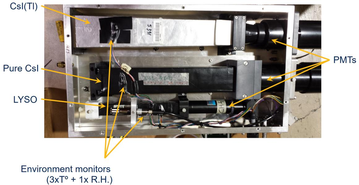
**Figure 4.5:** One calorimeter unit in Beast II. PMT: photomultiplier tube; T°: temperature sensor; R.H.: relative humidity sensor.
