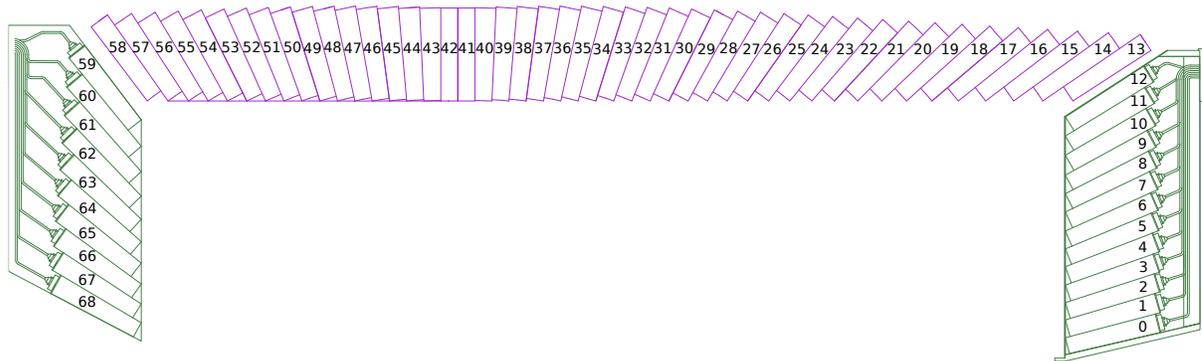
Figure 5.32: Mapping of the angular index  $\theta_{ID}$  in the ECL. The forward side of the detector is on the right of the figure. Figure reproduced from [79].
