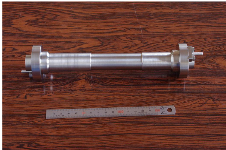
Figure 3.10: Current design of straight part of the beam pipe(top). The one-way cooling scheme is adopted. The mockup of the beam pipe with the one-way cooling system(bottom).
