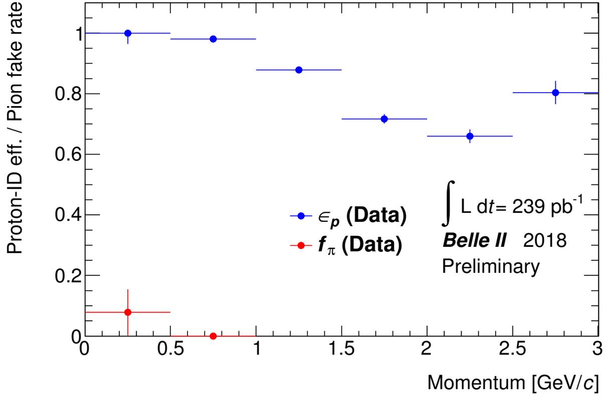
FIG. 4: This figure shows the proton-ID efficiency and the pion fake rate as a function of momentum by using combined PID for data. The proton-ID requirements are  $\mathcal{L}_{p/\pi} > 0.6$  and  $\mathcal{L}_{p/K} > 0.6$ . Further detail is described in BELLE2-NOTE-PH-2018-036.
