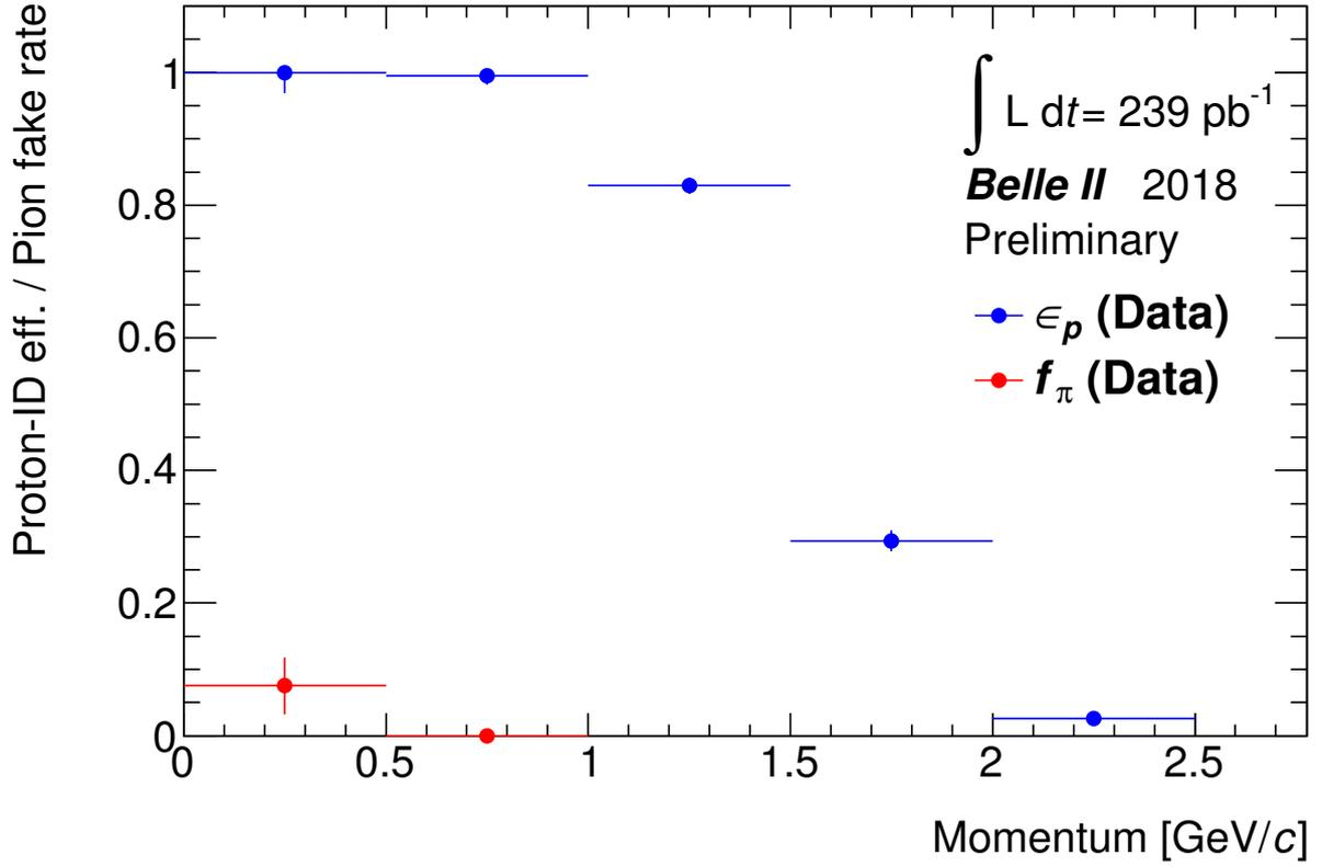
FIG. 6: This figure shows the proton-ID efficiency and the pion fake rate as a function of momentum by using CDC likelihood only for data. The proton-ID requirements are  $\mathcal{L}_{p/\pi}^{\text{CDC}} > 0.6$  and  $\mathcal{L}_{p/K}^{\text{CDC}} > 0.6$ . Further detail is described in BELLE2-NOTE-PH-2018-036.
