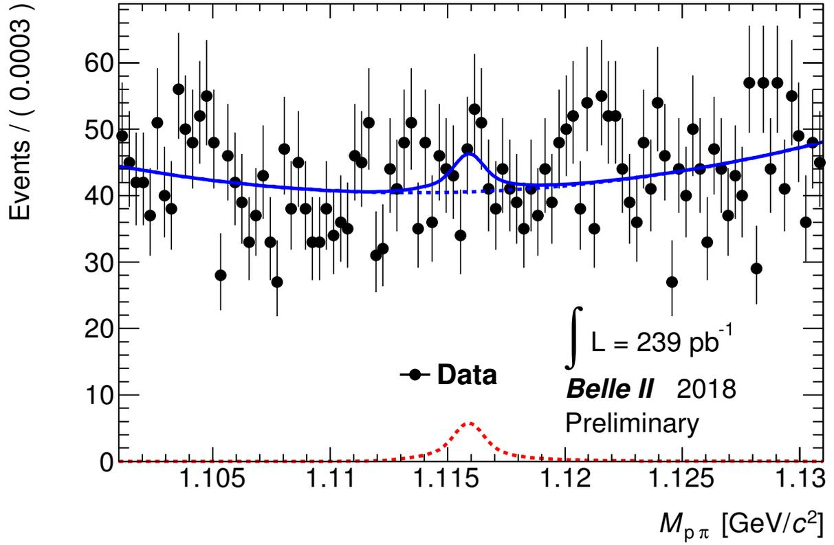
FIG. 3: This figure shows the  $p\pi$  invariant mass after a track assumed pion requires proton ID (right). The proton-ID requirements are  $\mathcal{L}_{p/\pi} > 0.6$  and  $\mathcal{L}_{p/K} > 0.6$ . For fit, the same p.d.f. as above are used. Here all parameters of the signal p.d.f. except number of the signal are fixed. Further detail is described in BELLE2-NOTE-PH-2018-036
