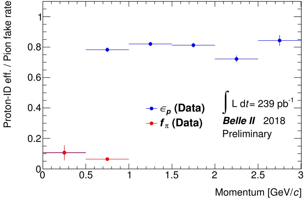
FIG. 5: This figure shows the proton-ID efficiency and the pion fake rate as a function of momentum by using TOP likelihood only for data. The proton-ID requirements are  $\mathcal{L}_{p/\pi}^{\text{TOP}} > 0.6$  and  $\mathcal{L}_{p/K}^{\text{TOP}} > 0.6$ . Further detail is described in BELLE2-NOTE-PH-2018-036.
