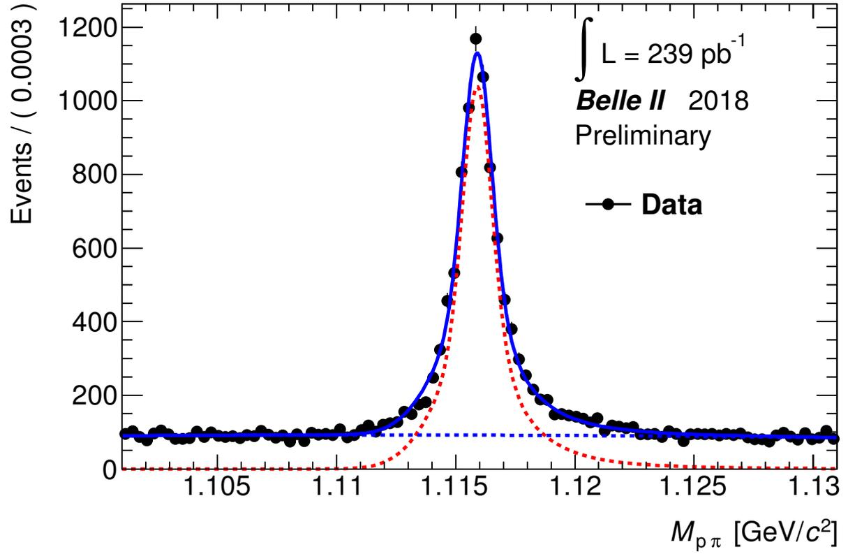
FIG. 2: This figure shows the  $p\pi$  invariant mass after a track assumed proton requires proton ID for data. The proton-ID requirements are  $\mathcal{L}_{p/\pi} > 0.6$  and  $\mathcal{L}_{p/K} > 0.6$ . For fit, the same p.d.f. as above are used. Here all parameters of the signal p.d.f. except number of the signal are fixed. Further detail is described in BELLE2-NOTE-PH-2018-036.
